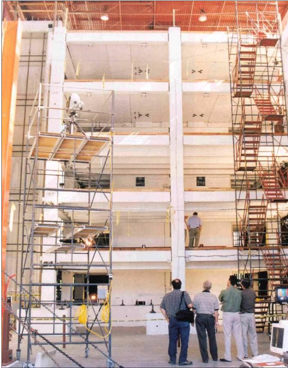
UC San Diego Test Facility – 60% Scale 5-Story Structure
