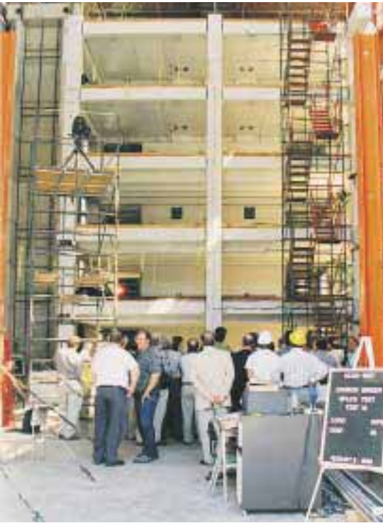
Rigorous tests performed last year on an experimental structure proved the success of the PRESSS program's connection techniques.
